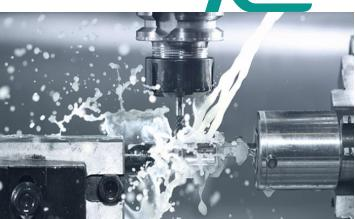
Metal cutting liquid contains fully-synthetic cutting fluid, semi-synthetic cutting fluid, emulsified cutting fluid, and oil cutting fluid. It's used to cool and lubricate the metal processing. Due to the high shear and functional additives, the foam is contributed. The unwanted foam can cause reservoir overflows, unplanned downtime and equipment damage.
